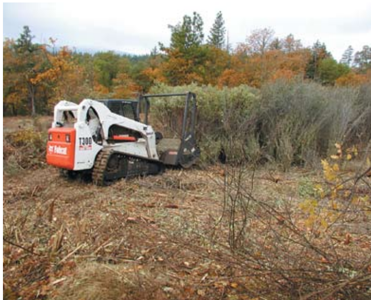
Figure 4. Brush Mulcher treating manzanita and wedgeleaf ceanothus brushfield in southwest Oregon. The cutting head, here mounted on a Bobcat-type tracked vehicle, efficiently cuts material up to 4 inches in diameter. Photo: Paul Howell.
